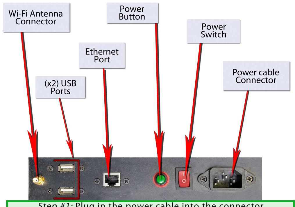
Step #1: Plug in the power cable into the connector Step #2: Flip the power switch to on position Step #3: Press on the power button to turn on the Kiosk
