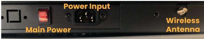
**Step 3:** After connecting the base to the screen, connect the power cord to the power input on the back of the base, plug the other end into an available power outlet and flip the main power switch to the on position. See previous image. (Note: Port layouts may vary depending on kiosk model but will still be similar. Main Power switch is shown in the "On" Position.)
